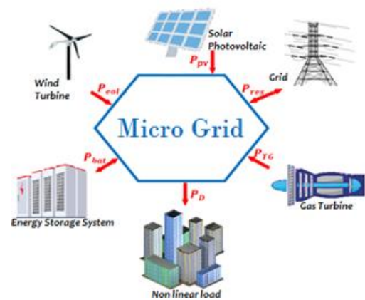
Figure: Studied MG overall architecture
