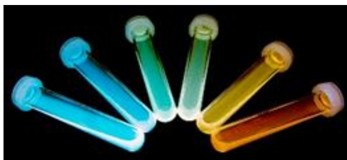
Fig. 1. The fluorescence of the carbon dots can be tuned from the blue to the far red/near-infrared regions of the spectrum.
