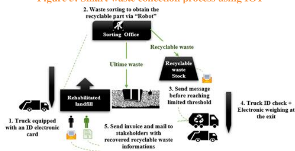
Figure 5: Smart waste collection process using IOT
