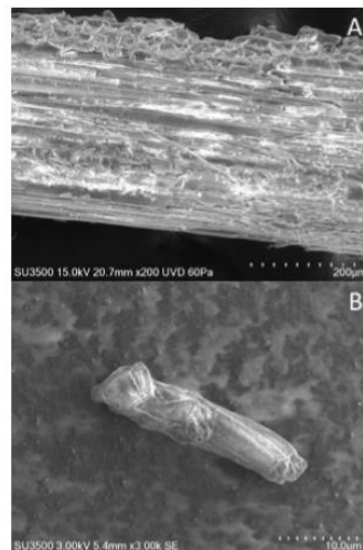
Figure 19. Morphological observations by SEM (A) bark tree of zalacca and (B) Nanocellulose. Figure adopted from Triyastiti et al. [47].
