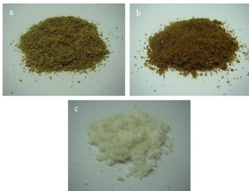
Figure 12. Photography of rice husk, Figures 12 (a), (b), and (c) are rice husk without treatment, rice husk treated with alkaline, and rice husks that have received alkaline and bleaching treatment, respectively. Figure adopted from Johar et al. [39].
