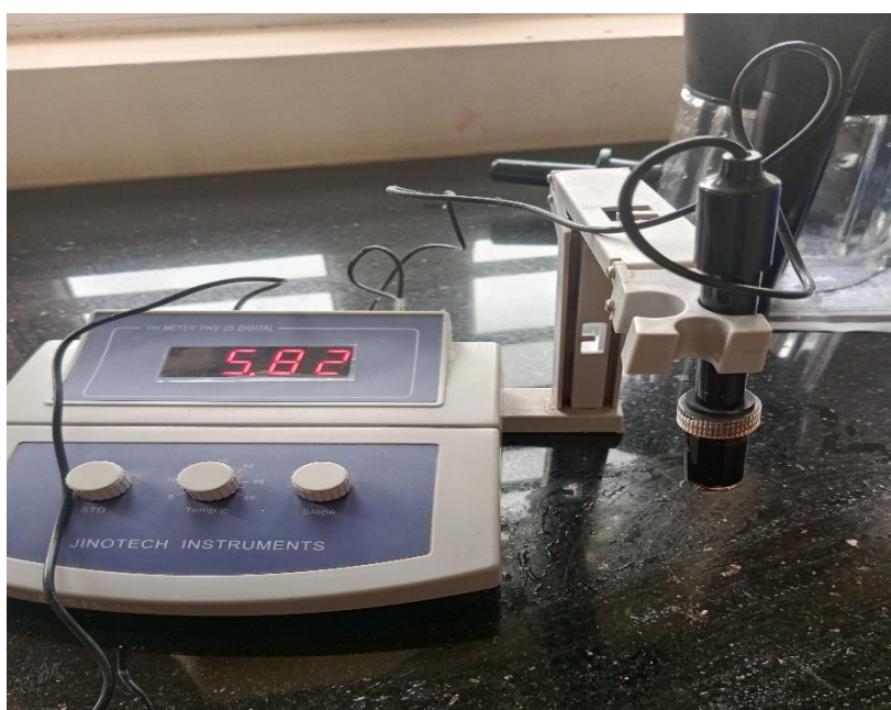
Figure 2.5 The pH procedure on the mixed sample
