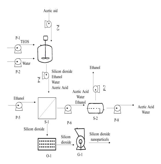
Fig 1: Flowchart diagram of the SiO<sub>2</sub> nanoparticle synthesis process
