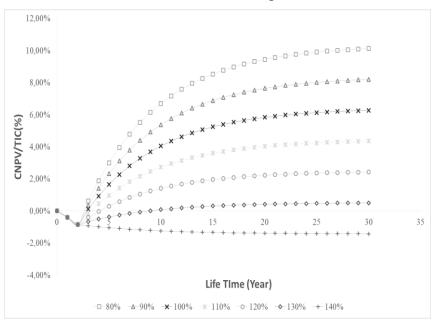
Fig 6. CNPV curves under various raw material prices
