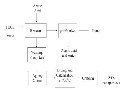
Fig 1. Flowchart of the SiO<sub>2</sub> nanoparticle synthesis process
