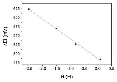
Fig. 2. Variation of  $\Delta E_i$  measured with  $R_i(H)$  in HF solution
