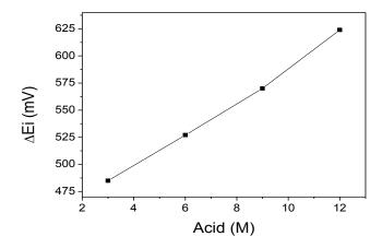
**Fig. 1**. Variation of  $\Delta E_i$  measured with HF concentration
